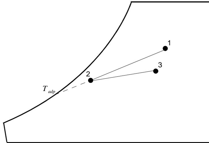
Process 1 – 2 represents the cooling in the coil. The air at the discharge of the coil (state 2) is used as supply air to the conditioned space. For a cooling coil, the air temperature at the discharge is a function of the bypass factor BF, the apparatus dew point  $T_{adp}$ , and the entering air temperature  $T_1$  :
